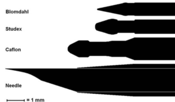
Diagram showing the differences in the the "cutting edge" of ear piercing studs used in piercing guns. The bottom silhouette is a single use hollow needle.
